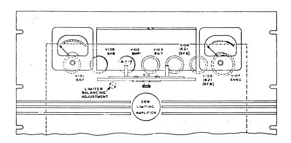
Figure 5-1. Tube Locating Diagram
